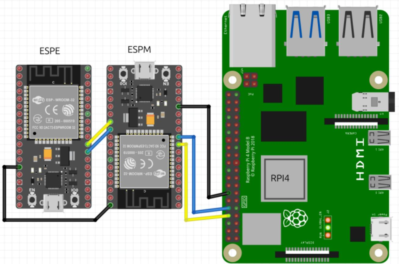
Raspberry Pi 4 → ESP32M ← ESP32E:
